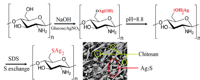
Scheme 1. Summary of experimental route for the synthesis of Chitosan/ \text{Ag}_2\text{S} nanocomposites.
